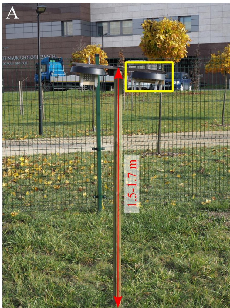
Fig. S2. A: View of the sampler located at about 150-170 centimetres above the ground level in the grassy area at the III Campus of the Jagiellonian University (Gronostajowa Street, Kraków, Poland – exact location in the Figure S1); B: Closer view (area marked with yellow rectangle) of the magnet matrix under the cover placed in order to protect from precipitations.
